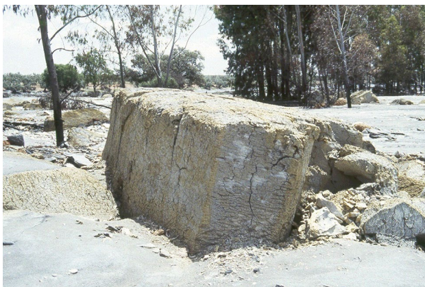
Fig. 7 Clay blocks ‘floating’ on the tailings flow. Note the parallelepipedic shape, sharp edges, and the joints covered by oxidation coatings
