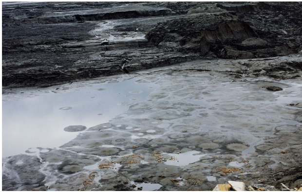
Fig. 14 Mud “volcanoes” observed a few hours after the failure on the surface of the depressed basin, upstream of the slid dam (Courtesy of J. M. Rodríguez Ortiz)
